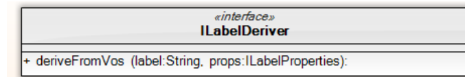
Figure 3.8: Interface responsible for the definition of methods needed to extract information from a specific label style.
