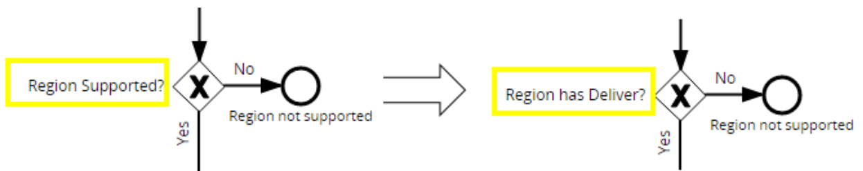
Figure 4.16: Process fragment which illustrates the scenario where an updated made to a Gateway description should also trigger an event description update.
