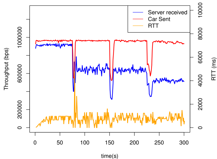
Figure 4.11: Throughput and RTT over the time in application E2 using Best effort approach
