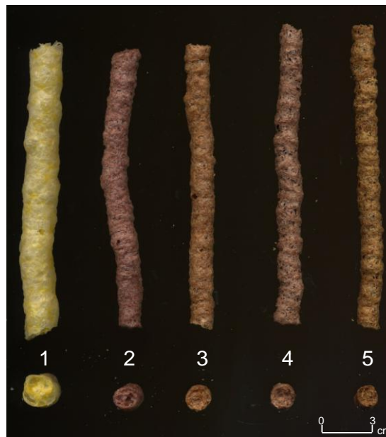
Fig. 5: Scanning materials obtained in extrusion processing with cross and longitudinal section, where: 1 = Control (corn); 2 = Sorghum BRS330; 3 = Sorghum BRS330+turmeric; 4 = Sorghum SC319; and 5 = Sorghum SC319+turmeric. The scale bar is 1:3 cm.
