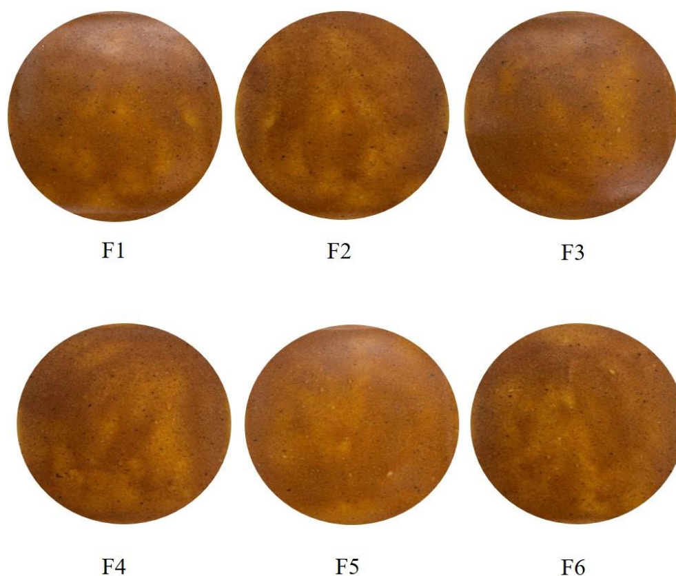
Figure 1. Visual aspects of the films: F1 (formulated using 1000 g kg -1 persimmon); F2 (formulated using 980 g kg -1 persimmon, 20 g kg -1 of OPF); F3 (formulated using 920 g kg -1 persimmon, 20 g kg -1 of OPF and 60 g kg -1 glycerol); F4 (formulated using 900 g kg -1 persimmon, 20 g kg -1 of OPF and 80 g kg -1 glycerol); F5 (formulated using 900 g kg -1 persimmon, 40 g kg -1 of OPF and 60 g kg -1 glycerol); and F6 (formulated using 880 g kg -1 persimmon, 40 g kg -1 of OPF and 80 g kg -1 glycerol).
