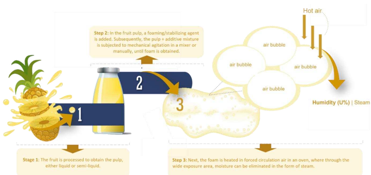
Figure 2 - Schematic model of foam layer drying.
