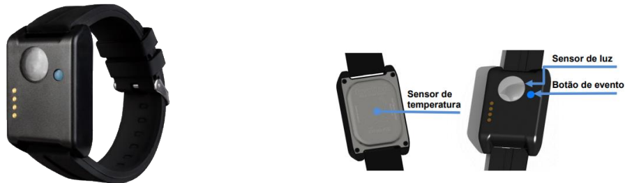
Figura 5 — ActTrust, Condor Instrument-Basic Mini Motion logger Actigraph®
